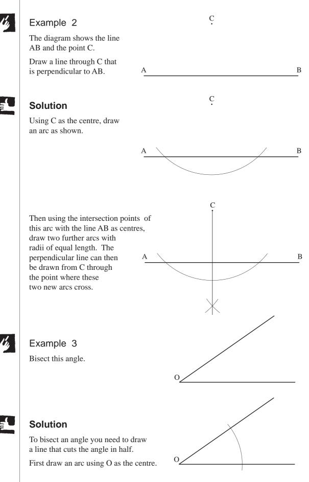
Then draw two further arcs of equal radius, using the points where the arc intersects the lines as the centres.
