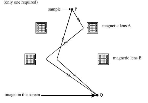
(ii) lens A: magnifies (or forms an intermediate image before B) (1) lens B: magnifies and focuses (or forms an enlarged image on the screen) (1)
